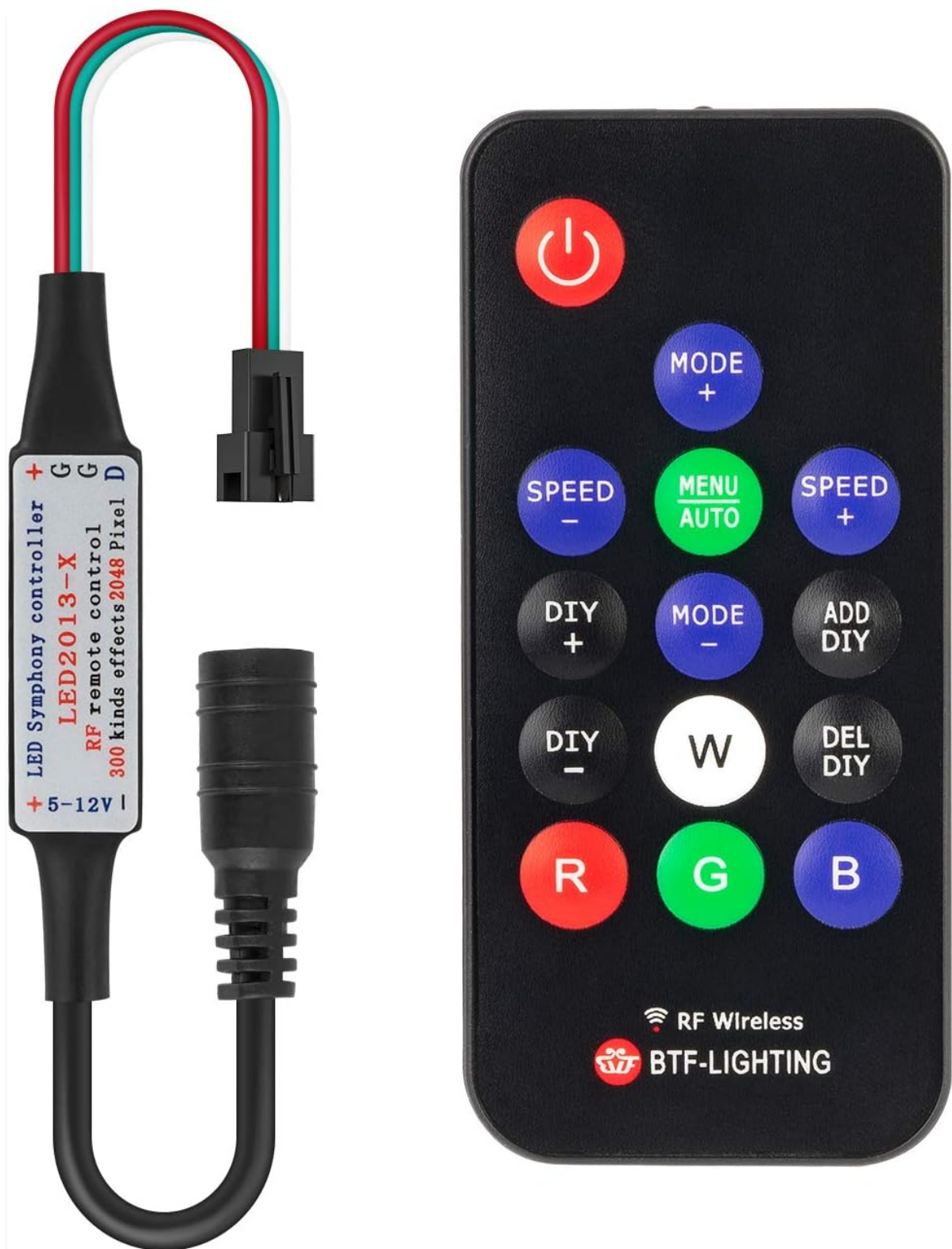
Image 3.1: The BTF-LIGHTING RF LED Controller and its accompanying 14-key remote control.
