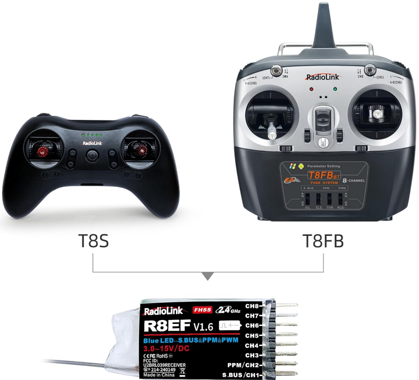
Image 4.1: The R8EF receiver is compatible with various Radiolink transmitters, including the T8S and T8FB models shown.
