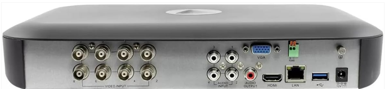
Image: Rear panel of the DVR, illustrating the video input (BNC), audio input/output (RCA), VGA, HDMI, LAN, USB, and power ports.
