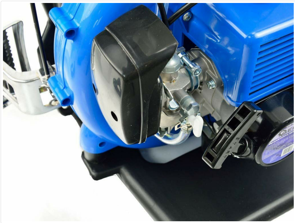
Figure 6.1: Detailed view of the engine's carburetor, an area that requires periodic inspection and cleaning for optimal performance.
