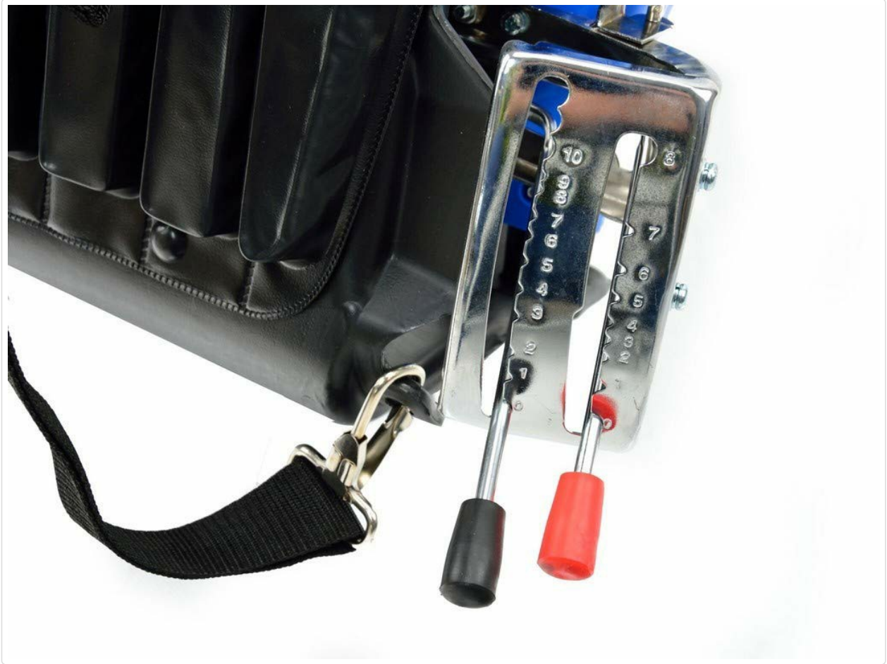
Figure 3.3: Detail of the control levers, typically used for adjusting throttle and material flow rate during operation.
