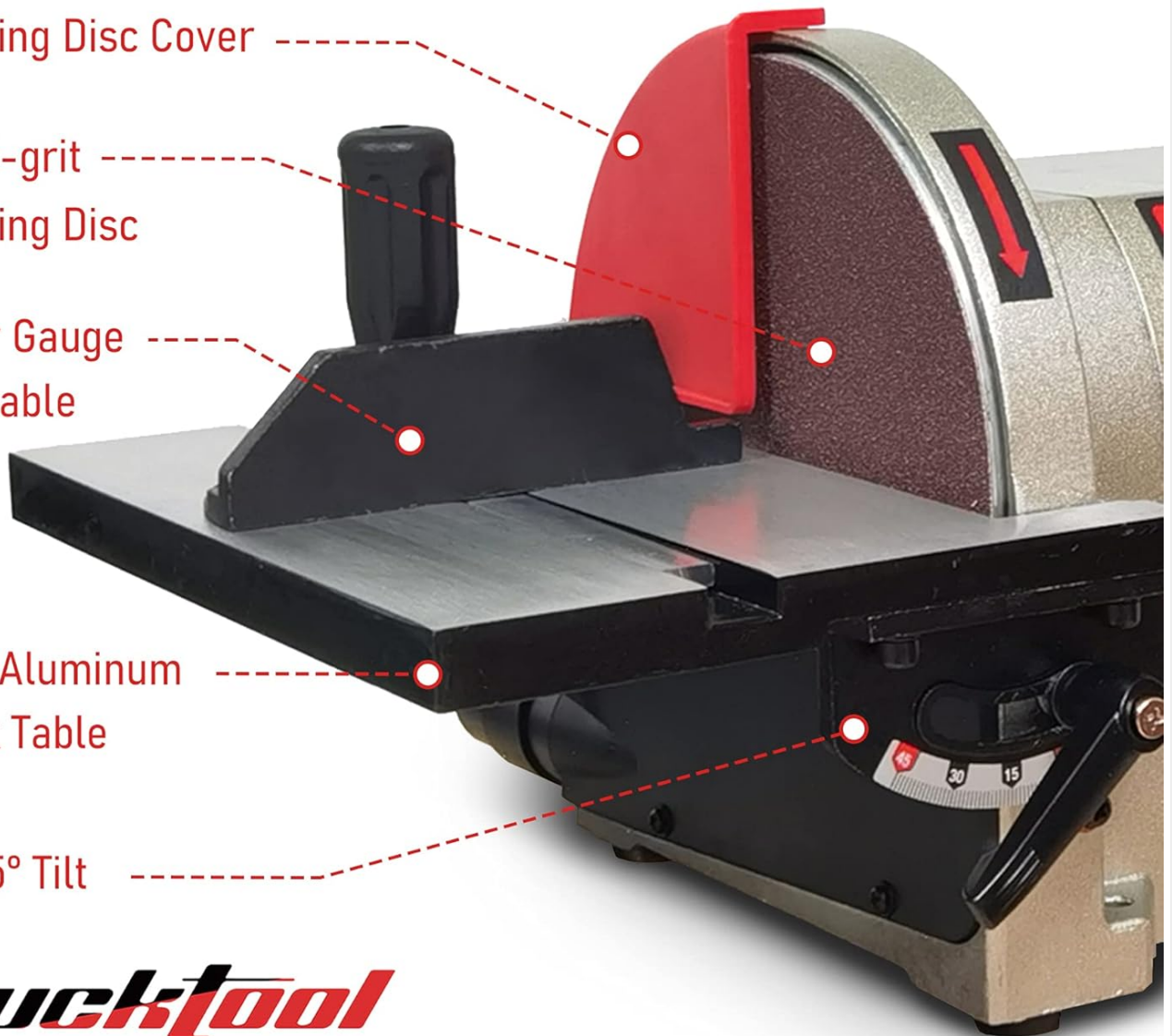
Figure 3.3: Detailed view of the disc sander components.
