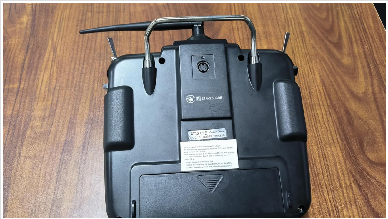
Image: Rear view of the Radiolink AT10II transmitter, showing the battery compartment and connection ports.
