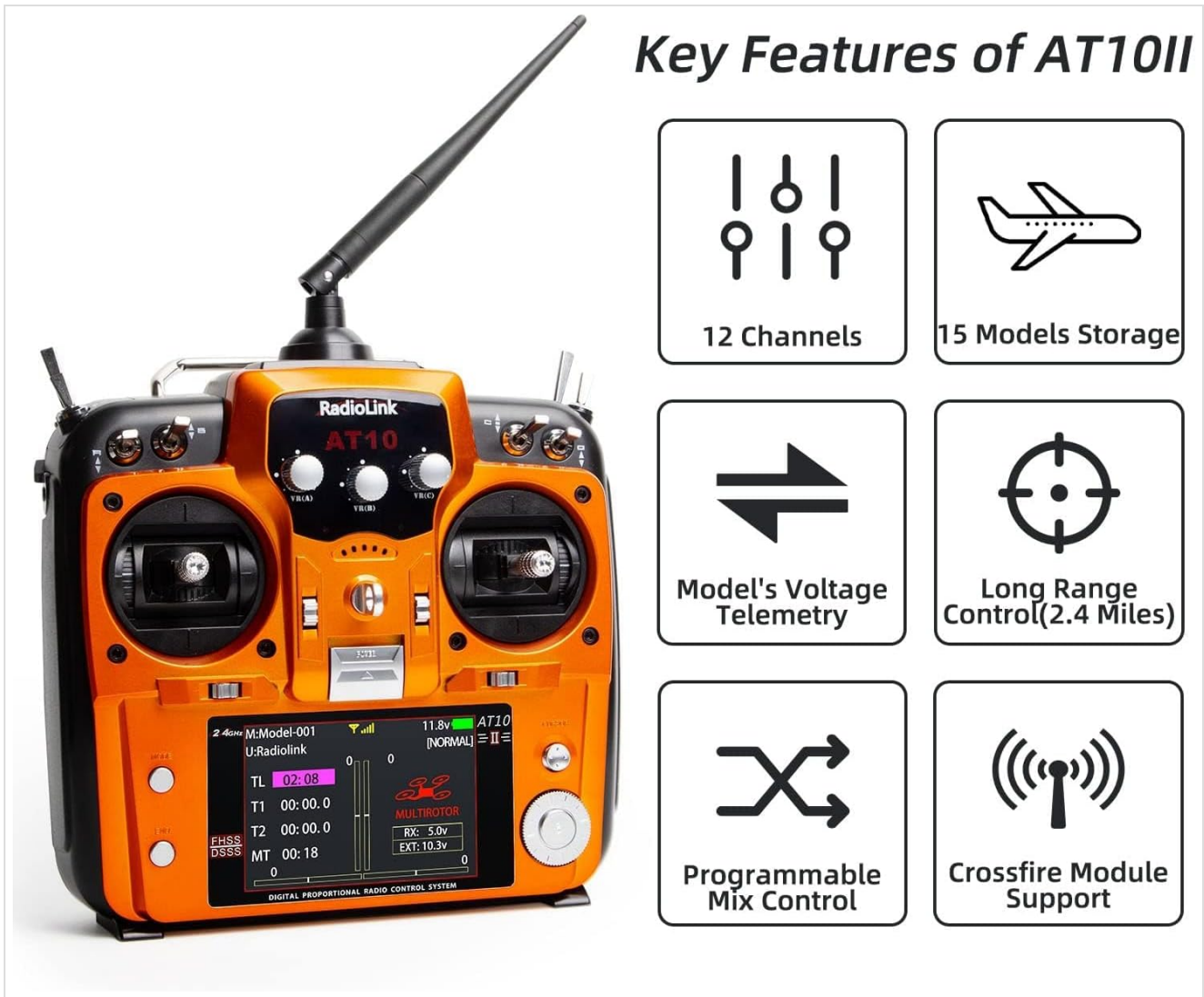
Image: Visual representation of the key features including 12 channels, 15 models storage, voltage telemetry, long-range control, programmable mix control, and Crossfire module support.
