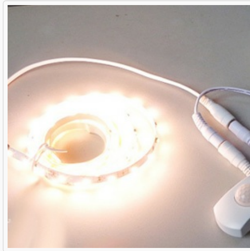
Figure 6.1: Sensor connected to an LED strip.
