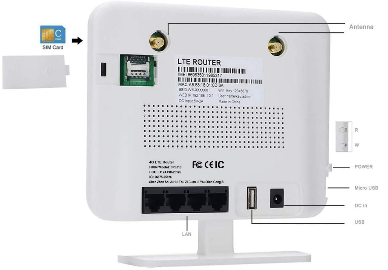
Figure 2.2: Back view of the KuWfi CPE810UT 4G LTE Router, highlighting the LAN ports, Micro USB, DC In, USB port, and external antennas.
