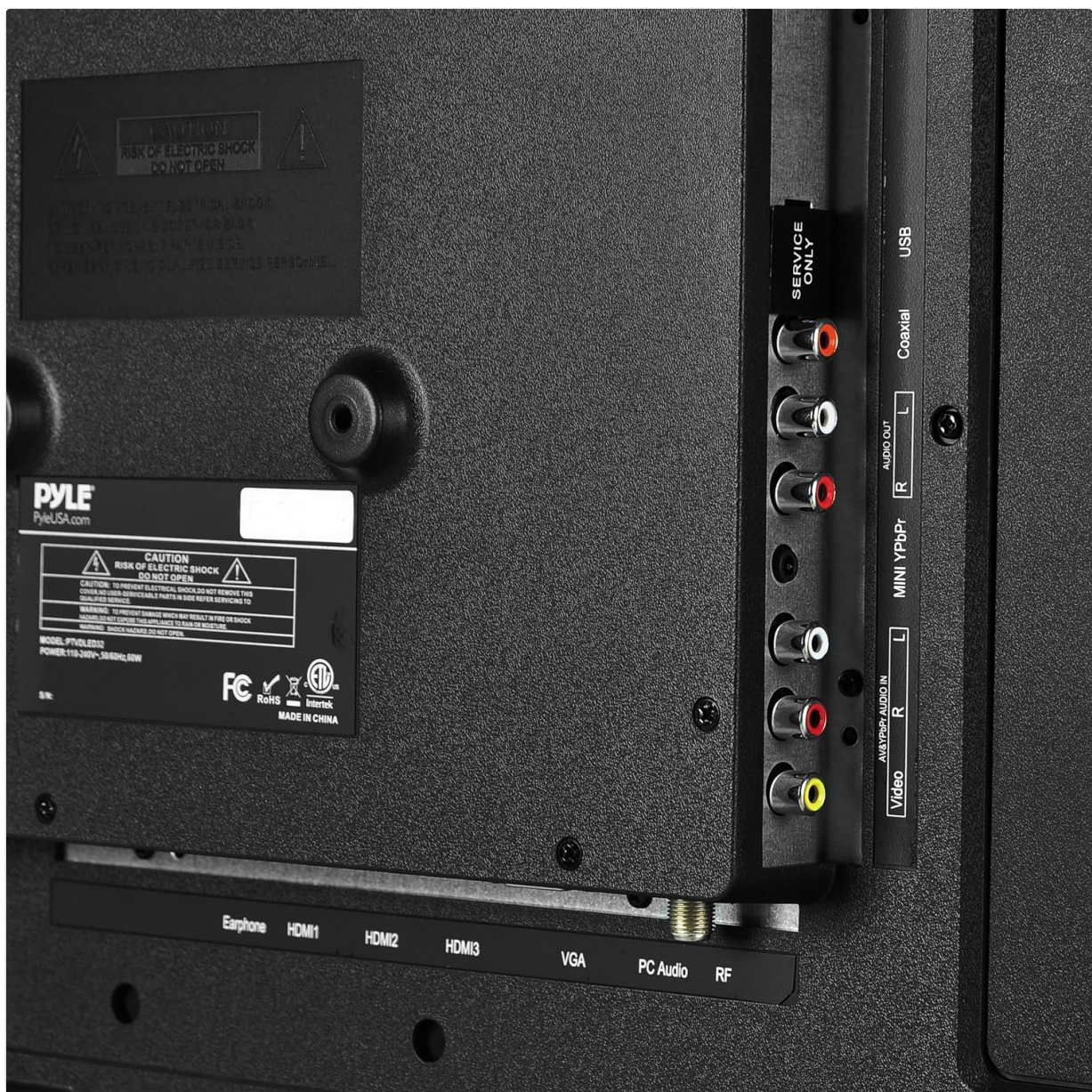
Image: Detailed close-up of the input/output ports on the Pyle 40 Inch LED TV, including HDMI, VGA, PC Audio, RF, Earphone, USB, Coaxial, Audio Out, Mini YPbPr, and Video/Audio In (RCA).
