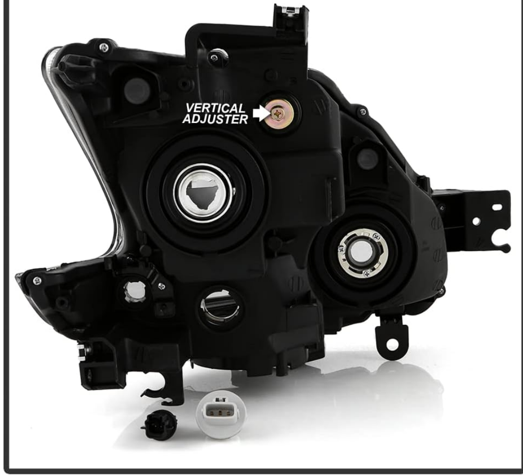
Figure 4.5: Location of the vertical adjuster screw. DO NOT OVER ADJUST!
