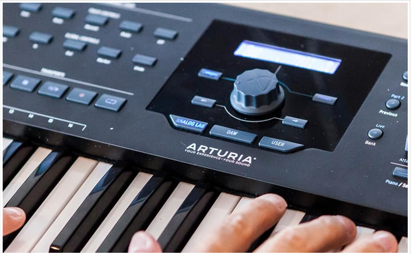
Image: A close-up view of the central control section of the Arturia KeyLab 61 MkII, showing the display screen, rotary encoder, and mode selection buttons (Analog Lab, DAW, User).
