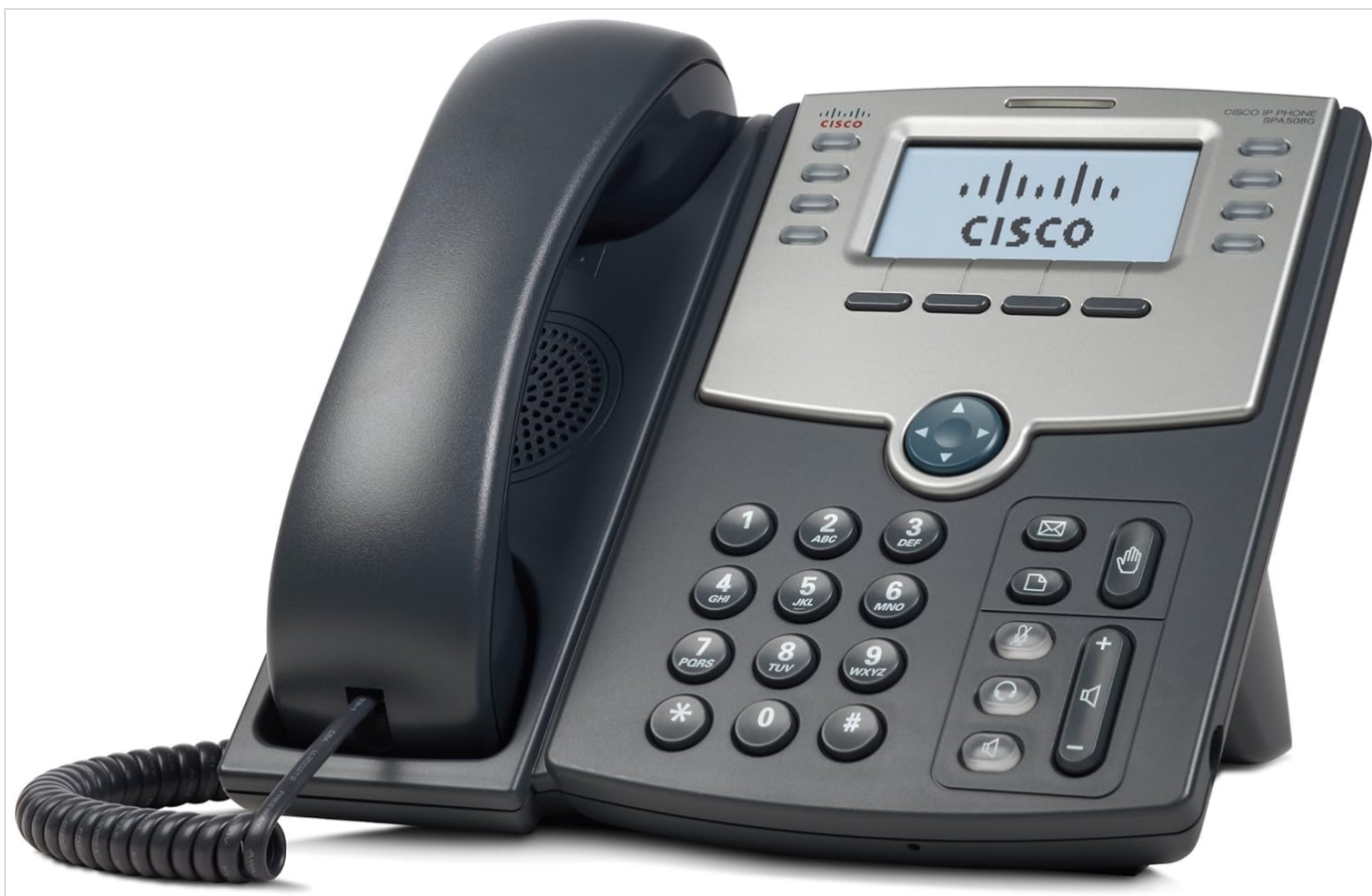
Figure 1: Cisco SPA 508G 8-Line IP Phone. This image displays the front view of the phone, highlighting its display, keypad, and function buttons. The handset is cradled on the left side, connected by a coiled cord.
