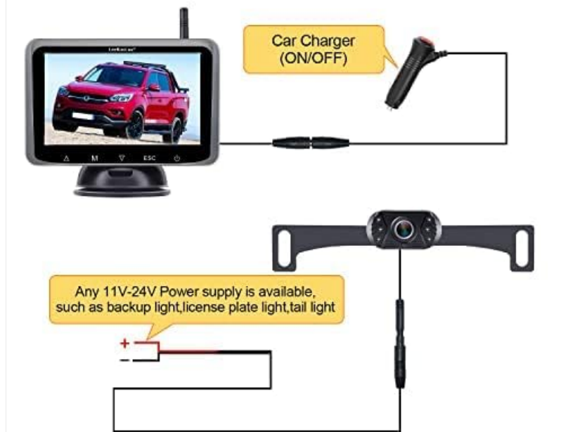
Image 2.1: Wiring diagram for the camera and monitor power connections.
