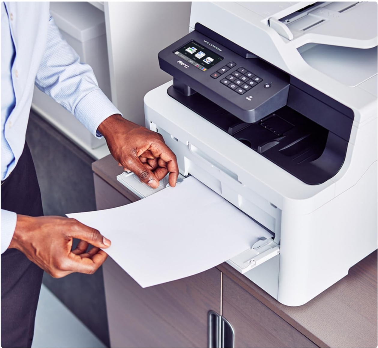
A user loading a single sheet of paper into the manual feed slot of the Brother MFC-L3750CDW printer.
