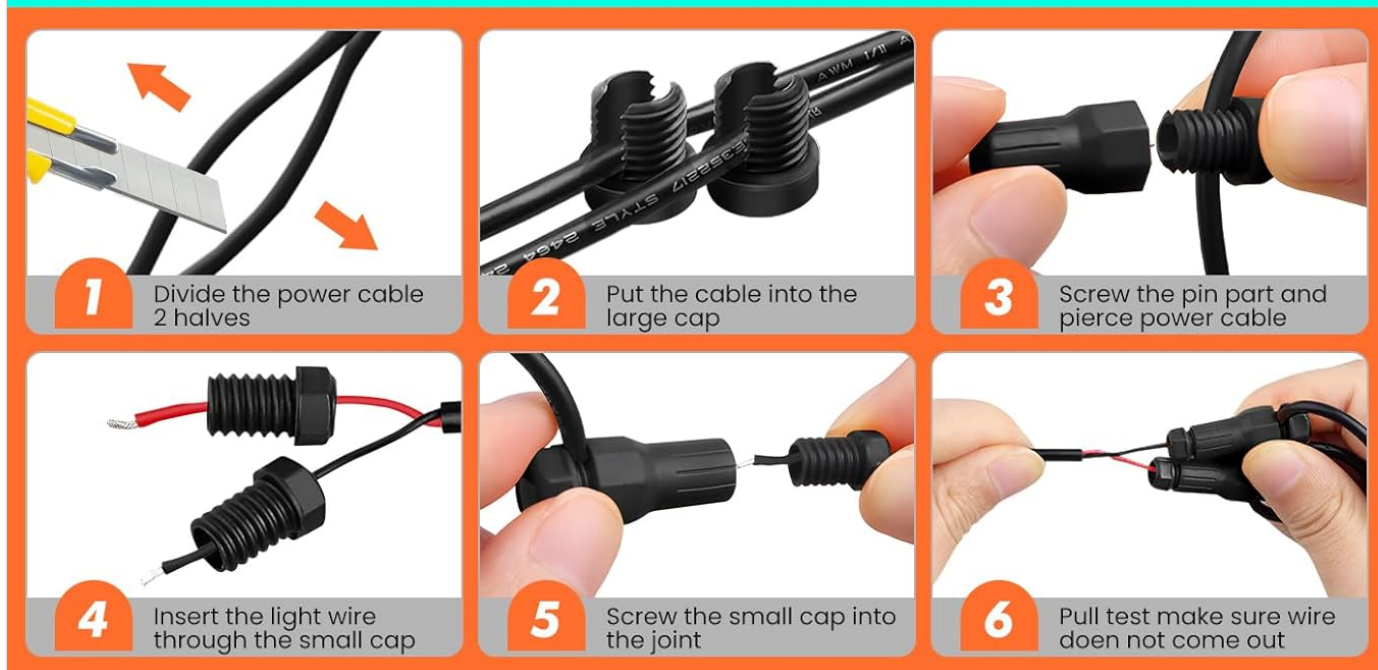
Figure 4.1: Step-by-step guide for connecting the low-voltage wires using the included connectors.
