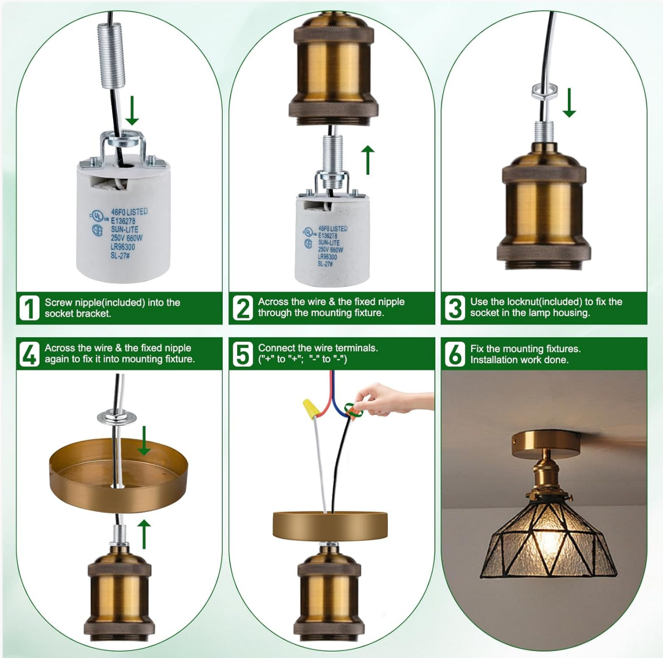
Image: Step-by-step installation process for the E26 light socket.
