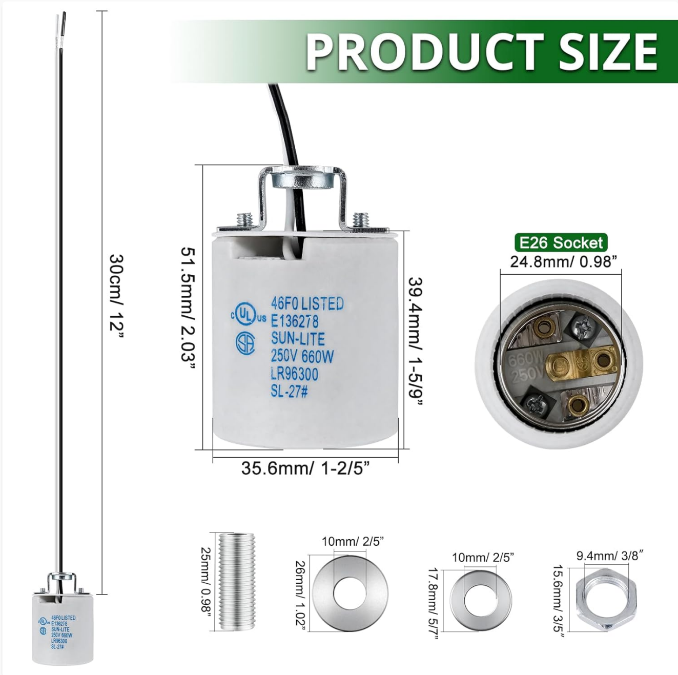
Image: Detailed product dimensions for the E26 socket and included hardware.
