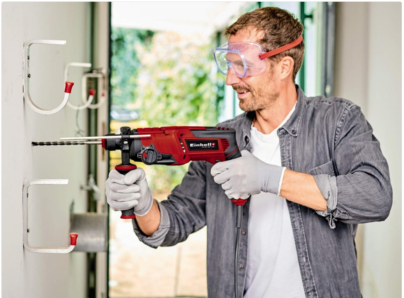
Figure 4: The adjustable depth stop and auxiliary handle, crucial for precise and controlled drilling.
