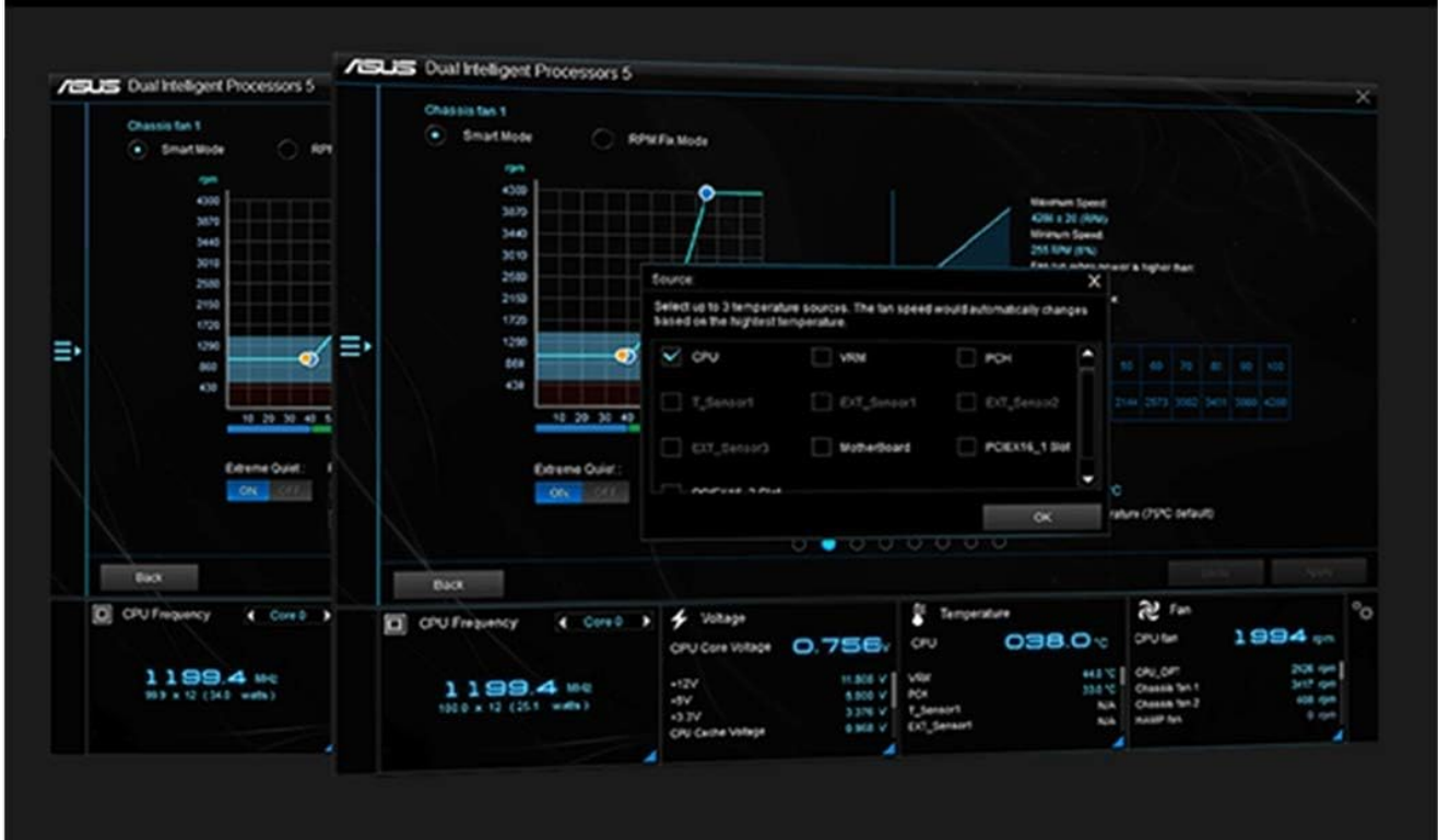
Figure 5.2: FanXpert 4 Core interface for flexible control of air and liquid cooling, with one-click intelligent tuning.
