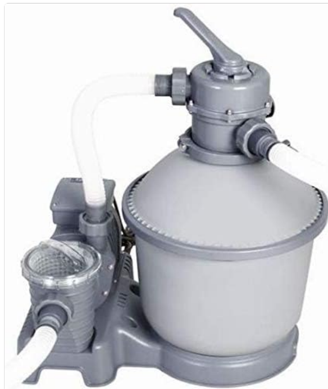
Image 3.1: The included Bestway Sand Filter Pump. This unit is responsible for circulating and filtering the pool water, removing debris and impurities. It features a multi-port valve for various functions like filtering, backwashing, and rinsing.
