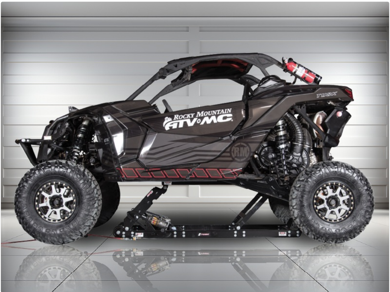
Figure 4: A UTV elevated to its maximum height on the Tusk UTV Lift, ready for maintenance.
