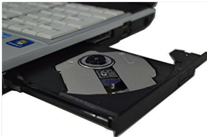
Image: A side view of the Fujitsu LIFEBOOK E741 laptop with its optical drive tray extended, showing the disc spindle.
