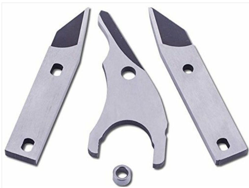
Figure 1: JTEX 18-Gauge Shear Cutter Replacement Blades. This image displays the complete set of replacement blades for the 18-gauge shear cutter. It includes two fixed blades (left and right), one movable blade, and a small bushing, all made of Cr5MOV1 material.
