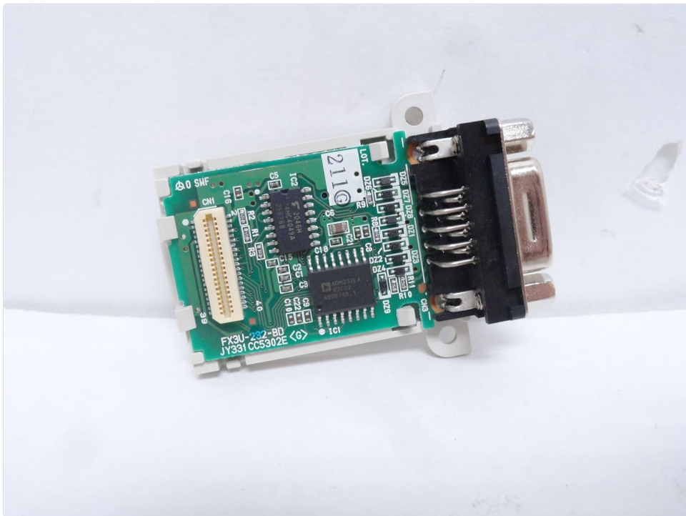
Figure 4: Top-down view of the Mitsubishi FX3U-232-BD module, showing the circuit board, connector, and mounting holes.
