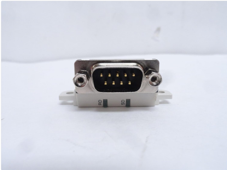
Figure 5: Front view of the Mitsubishi FX3U-232-BD module, focusing on the 9-pin D-sub (RS-232) connector.
