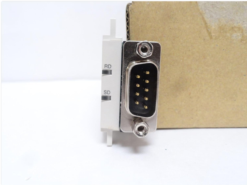
Figure 6: Side view of the Mitsubishi FX3U-232-BD module, showing the RS-232 connector and the module's profile.
