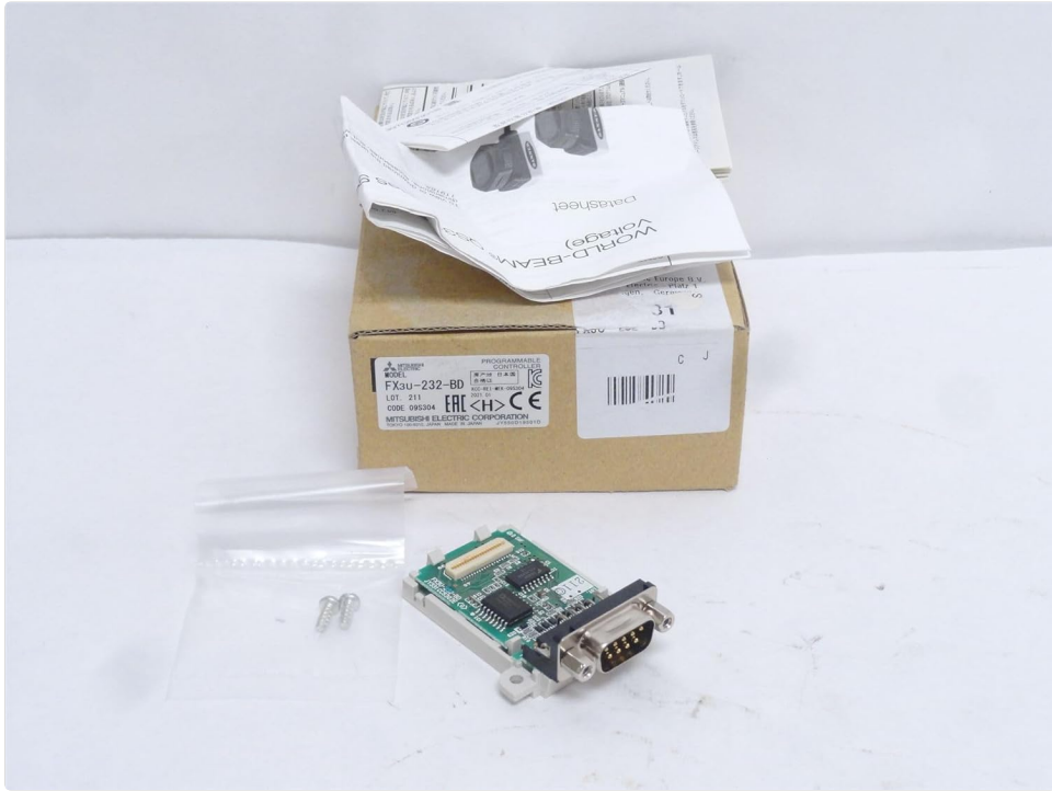
Figure 1: Mitsubishi FX3U-232-BD communication expansion board in its original packaging, alongside the board itself and small screws.
