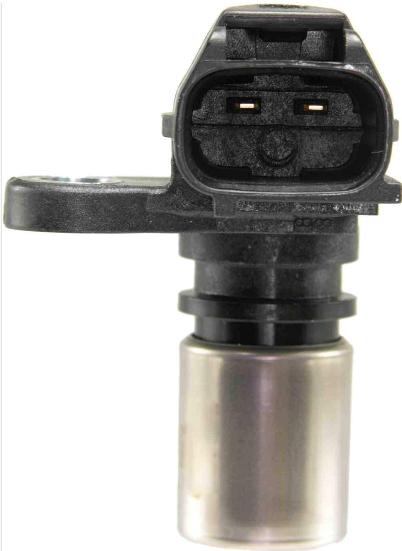
Figure 2: Side view of the NTK Crankshaft Position Sensor EH0320, showing the mounting tab and electrical connector orientation.
