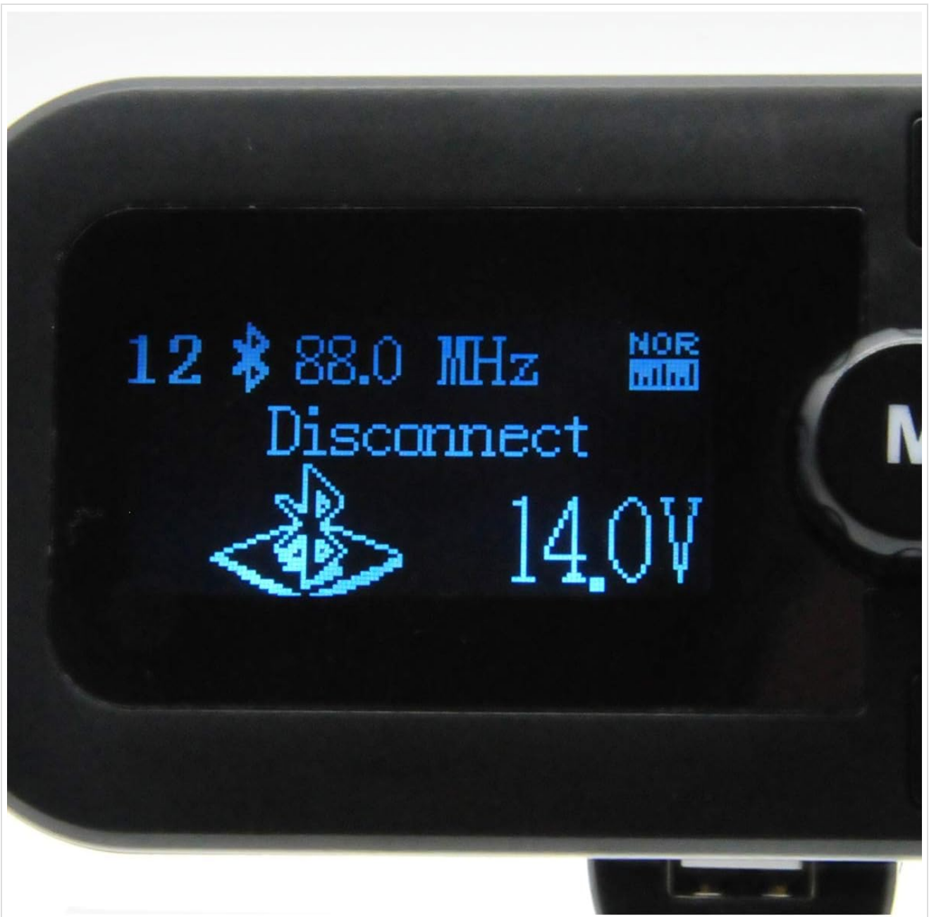
Image: A close-up of the MobileSpec FM Transmitter's LED display, showing the Bluetooth connection status (indicating 'Disconnect'), the current FM frequency, and the vehicle's battery voltage (14.0V), providing key operational information.
