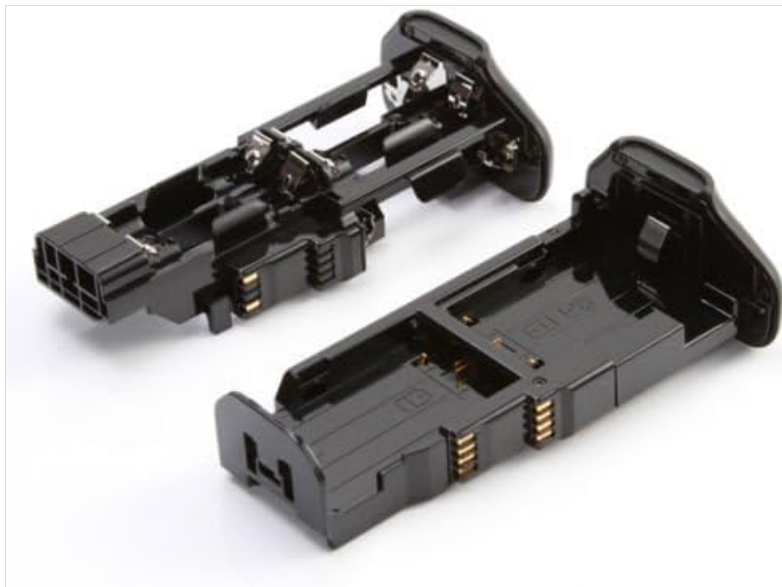
Figure 3: The AA battery magazine (left) and the Li-ion battery magazine (right) for the Meike MK-7DR II PRO Battery Grip.
