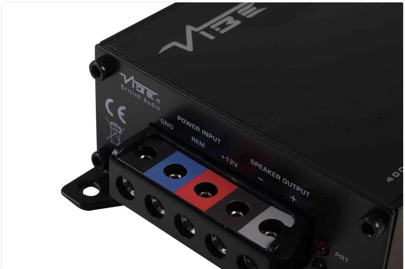
Figure 5.1: Detailed view of the power input and speaker output terminals. From left to right: GND (Ground), REM (Remote Turn-On), +12V (Power Input), and Speaker Output (+/-).
