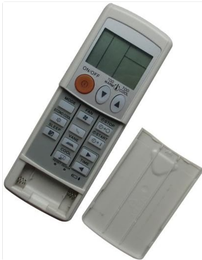
Image: The remote control with its battery cover removed, revealing the two AAA battery slots. This illustrates where to insert the batteries.
