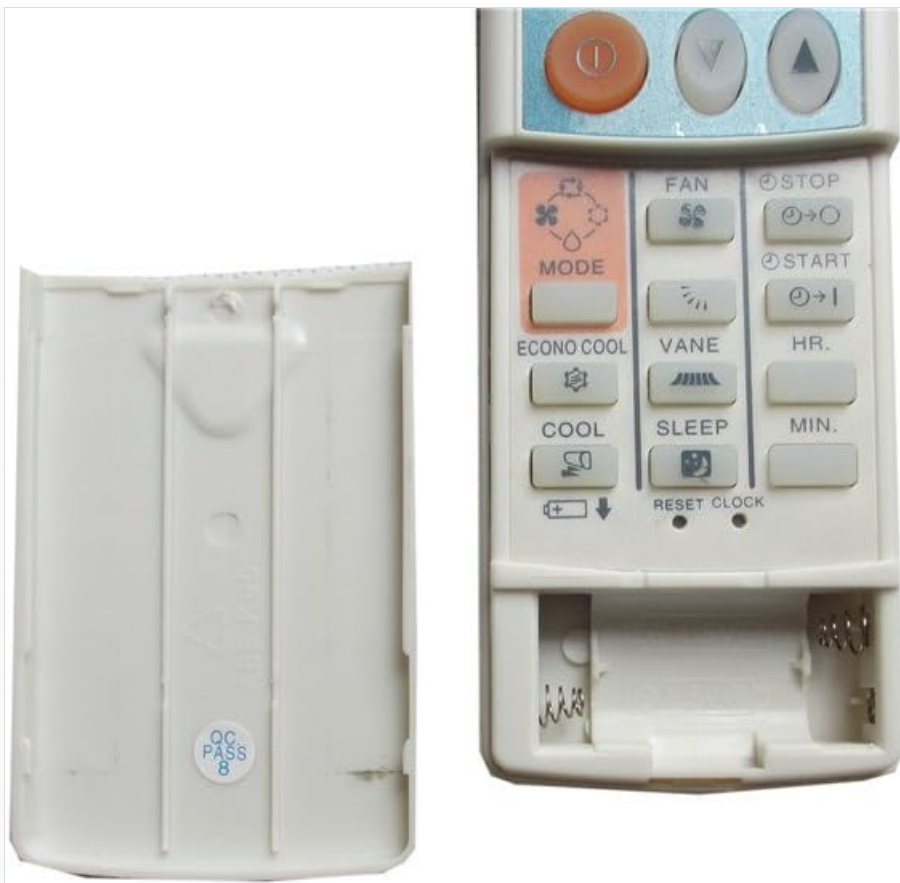
Image 2: Rear view of the Easytry123 replacement remote control with the battery compartment cover removed. This image illustrates where the two AAA batteries should be placed.
