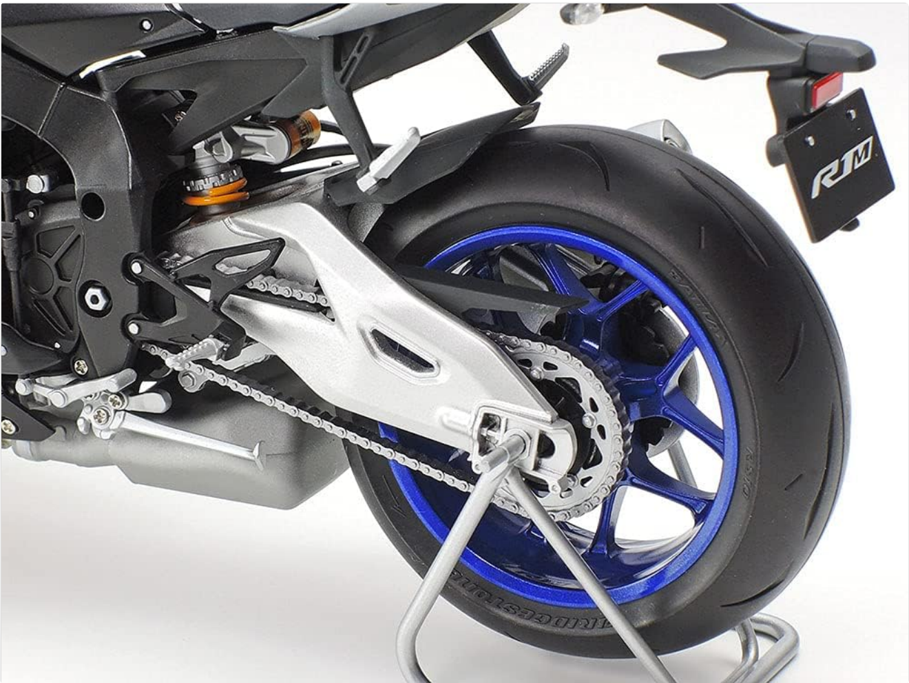
Image: Detailed view of the rear wheel, chain, and swingarm of the assembled model, highlighting the intricate mechanical details.
