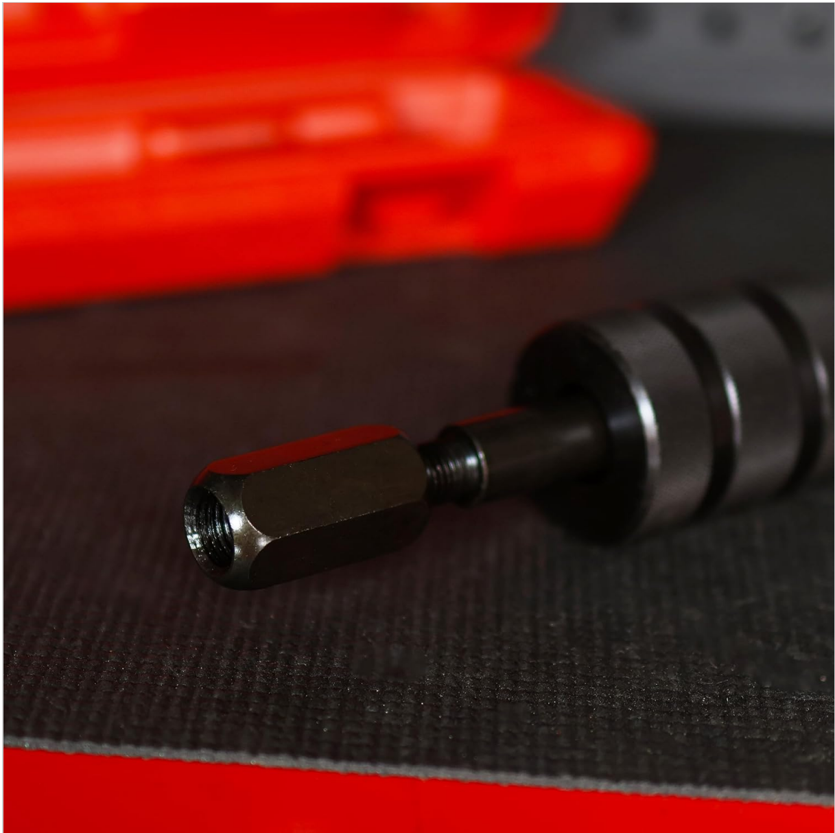
Image 3: Close-up view of a threaded adapter attached to the puller tool.
