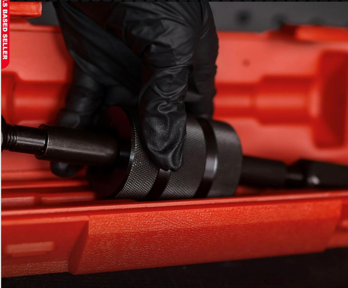
Image 4: Demonstration of using the slide hammer mechanism for injector removal.
