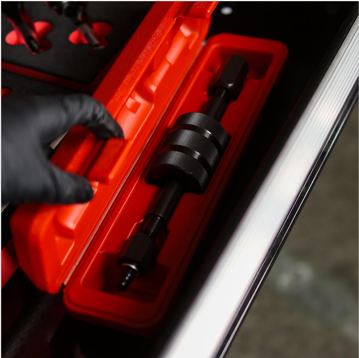
Image 5: Storing the ABN Diesel Injector Puller Tool in its protective case after use.
