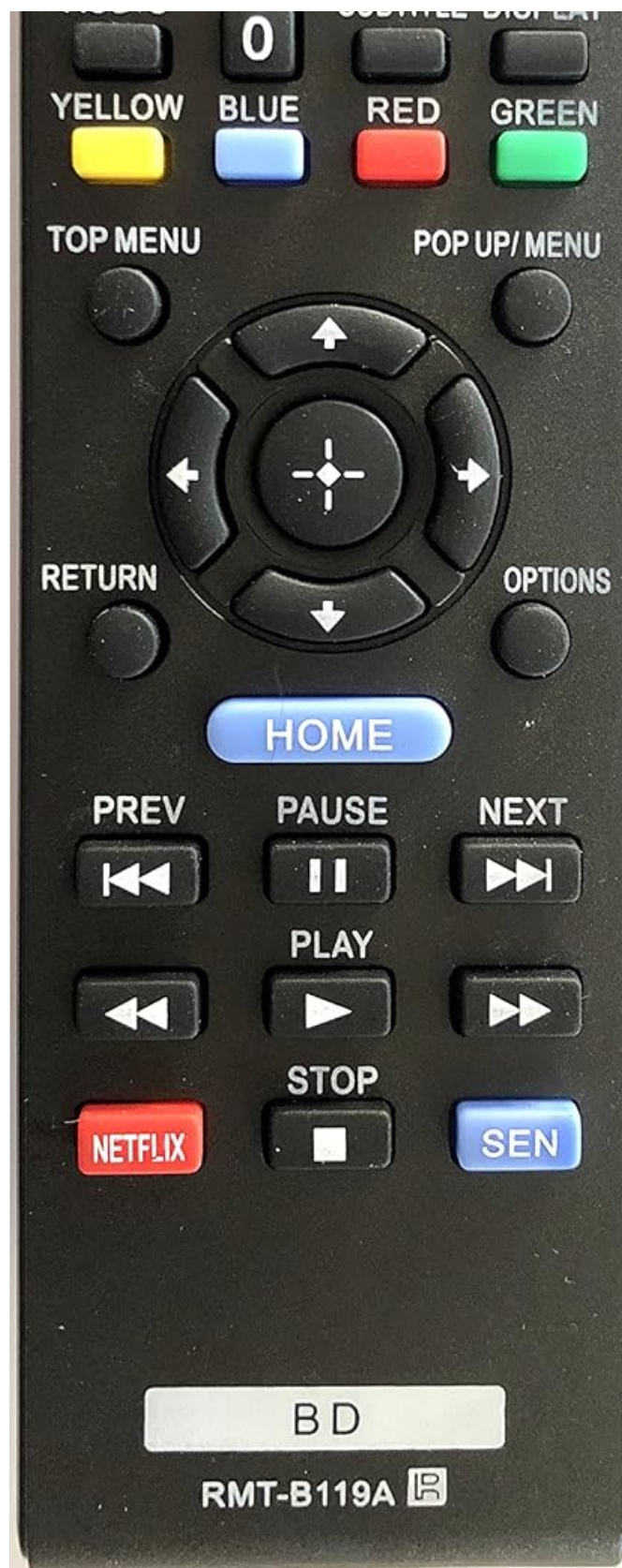
Image 1: Front view of the USARMT RMT-B119A replacement remote control, showing all buttons including numeric keypad, navigation, playback controls, and dedicated Netflix and SEN buttons.
