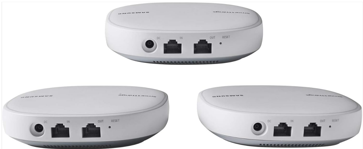
Figure 1.2: Rear view of three Samsung SmartThings Mesh Routers, highlighting the DC power input, IN (WAN) Ethernet port, OUT (LAN) Ethernet port, and a Reset button on each unit.
