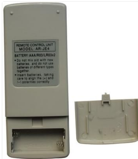
Figure 1: Rear view of the remote control with the battery compartment open, illustrating where to insert AAA batteries.
