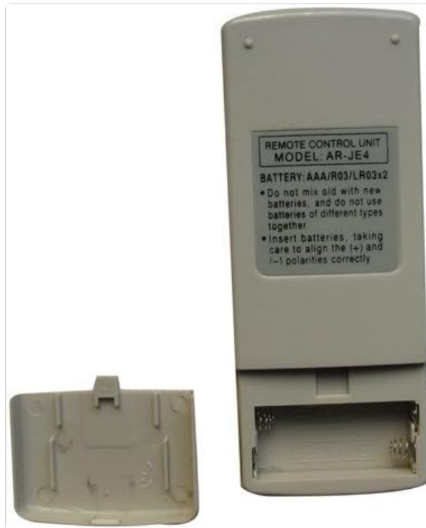
Figure 1: Rear view of the remote control with the battery cover removed, illustrating the battery compartment and polarity markings. The label indicates "REMOTE CONTROL UNIT MODEL: AR-JE4" and "BATTERY: AAA/R03/LR03x2".
