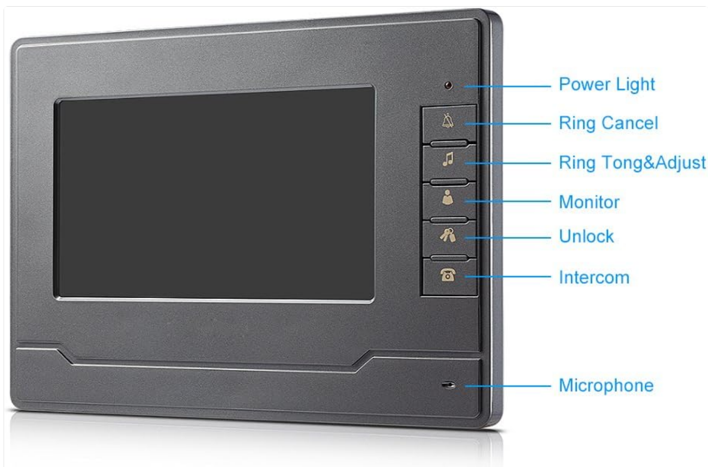
Figure 3.1: Indoor Monitor Components
