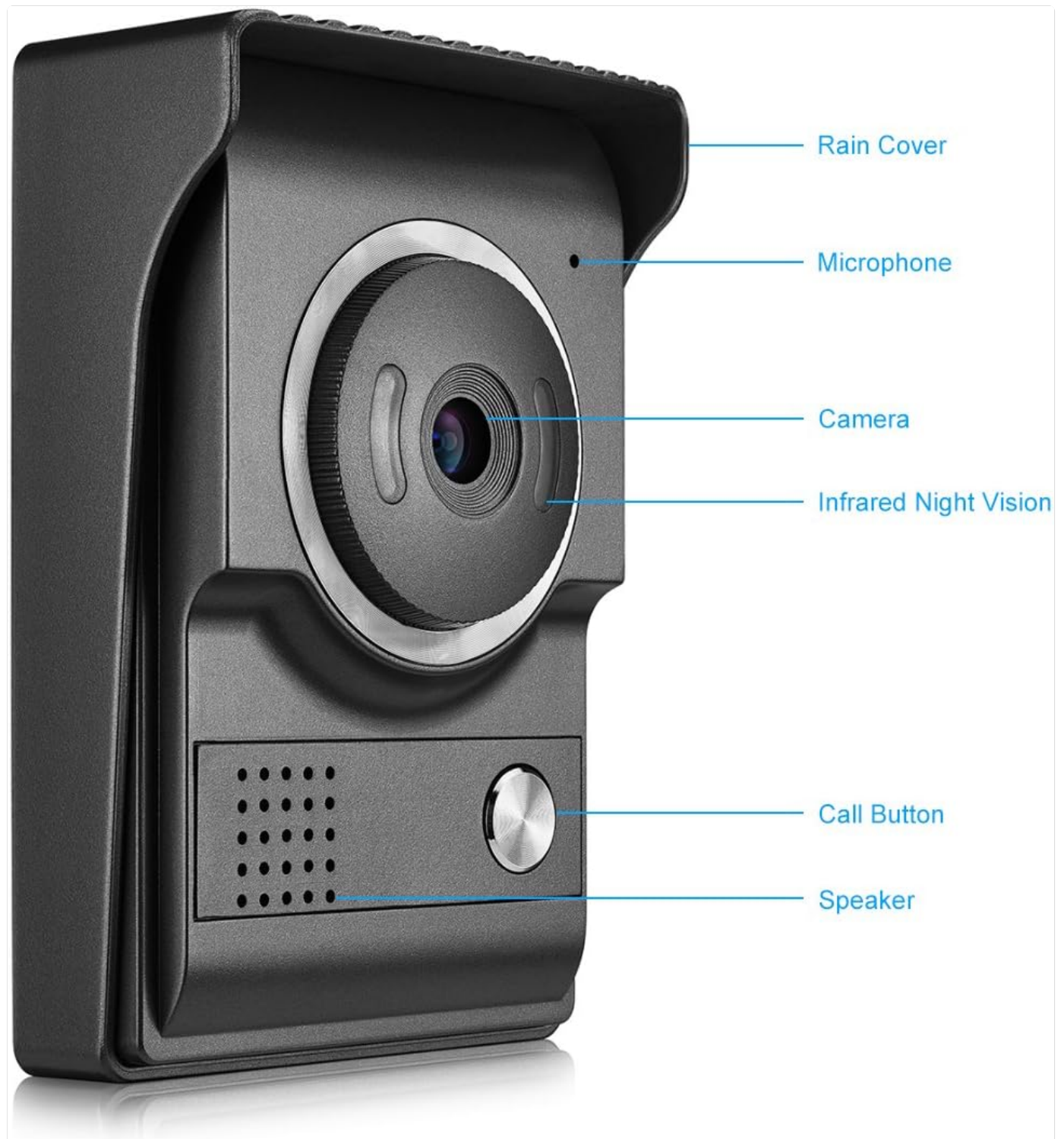
Figure 3.3: Outdoor Doorbell Unit Components
