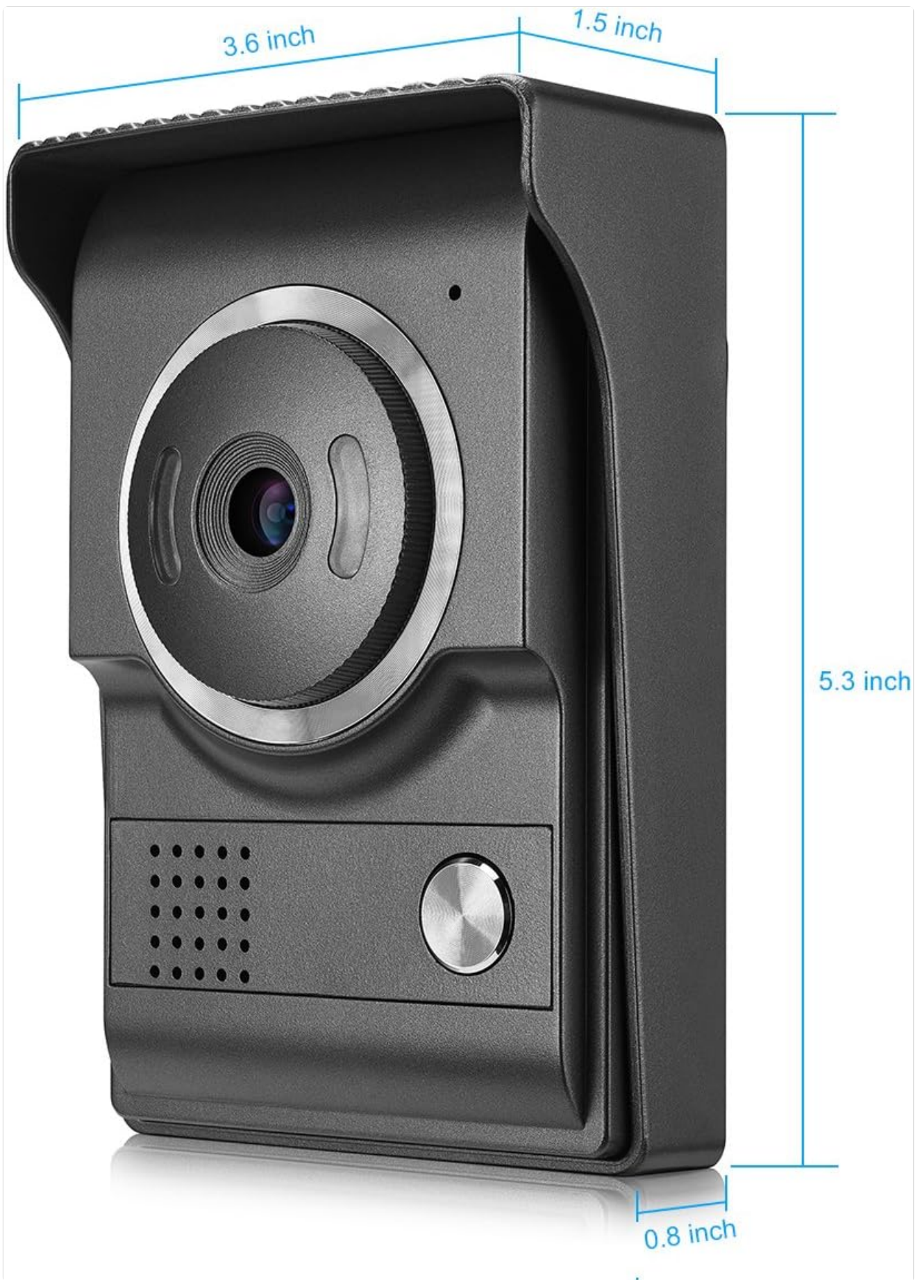
Figure 3.4: Outdoor Doorbell Unit Dimensions
