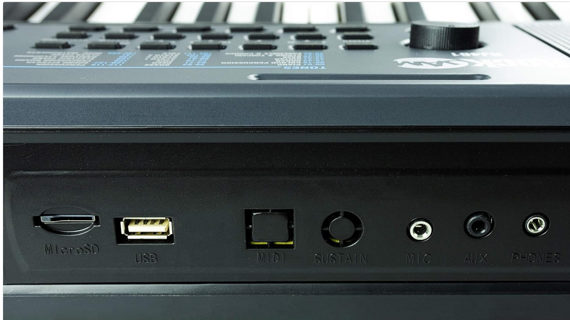
Figure 7: Connectivity ports for various external devices.
