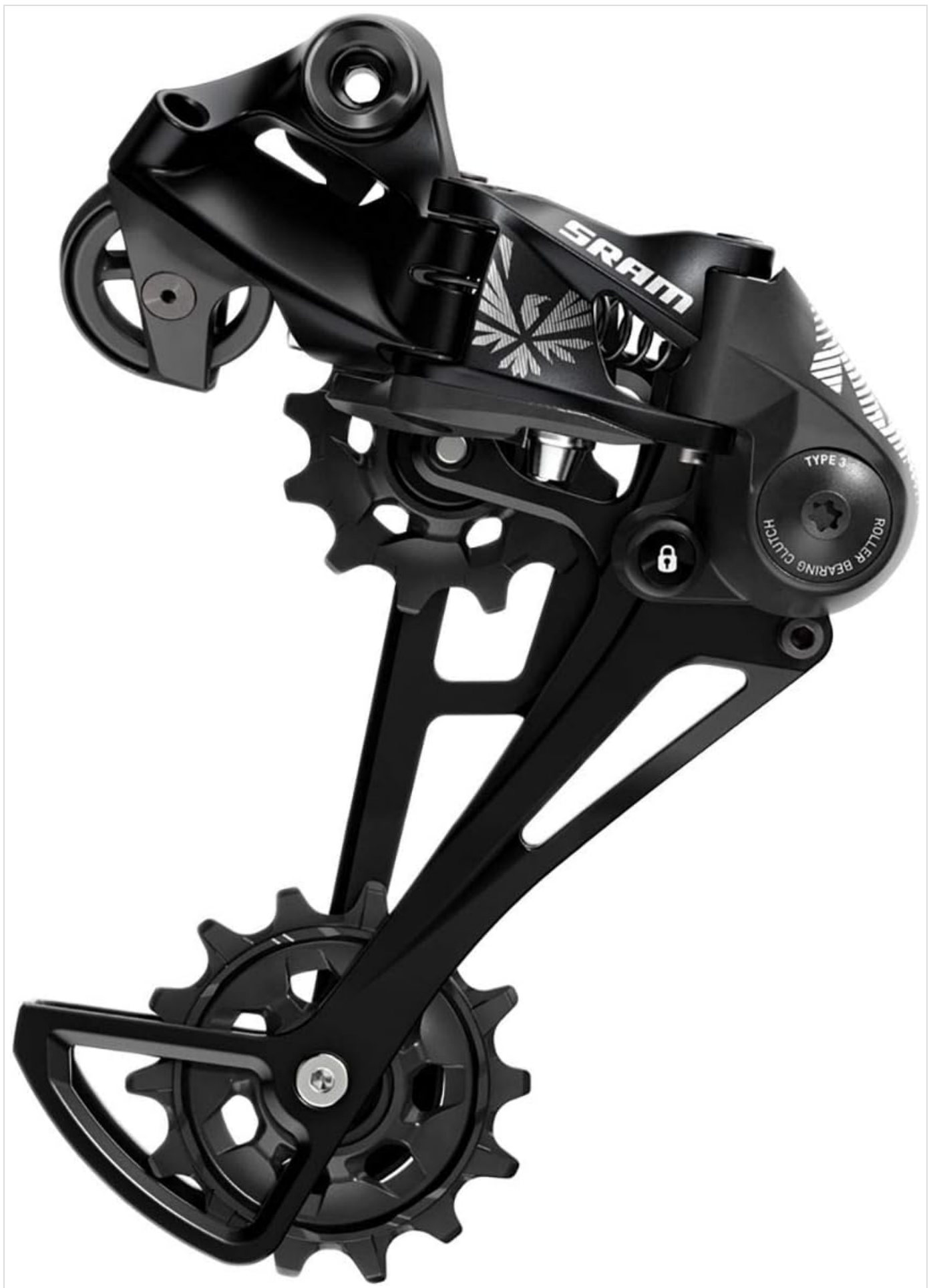
Image 5.1: The SRAM NX Eagle rear derailleur, a critical component for smooth shifting and a common point for troubleshooting adjustments.
