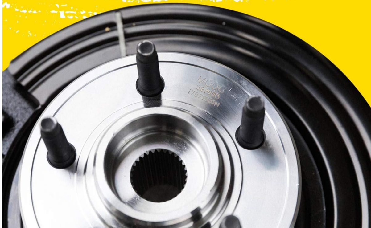
Figure 1: The MOOG LK009 assembly is designed for easy, bolt-on installation, reducing the need for specialized tools.
