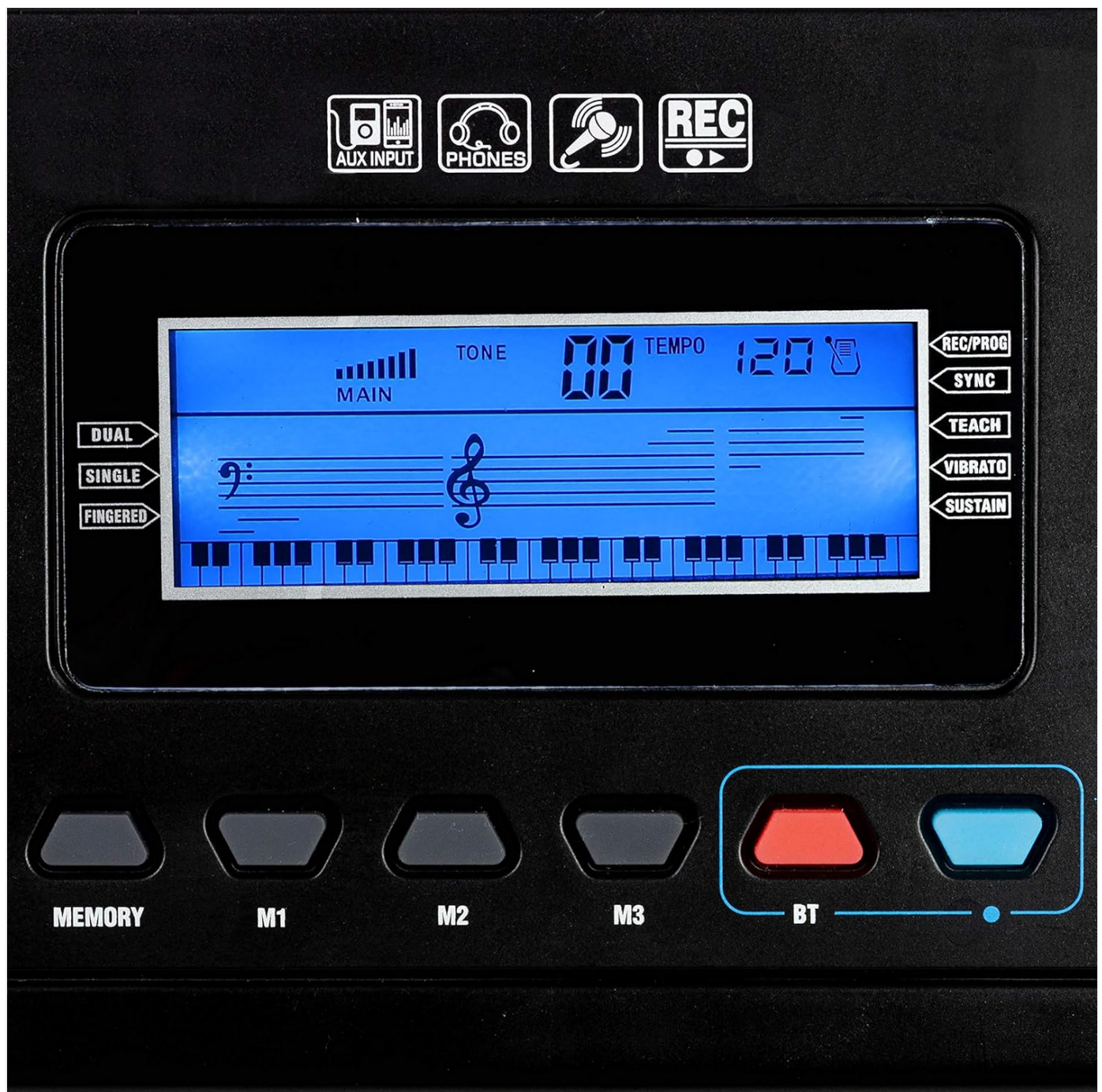
Figure 4.2: Detailed view of the LCD display showing current settings like tone and tempo, along with buttons for Memory, Bluetooth (BT), and various playback/recording functions.
