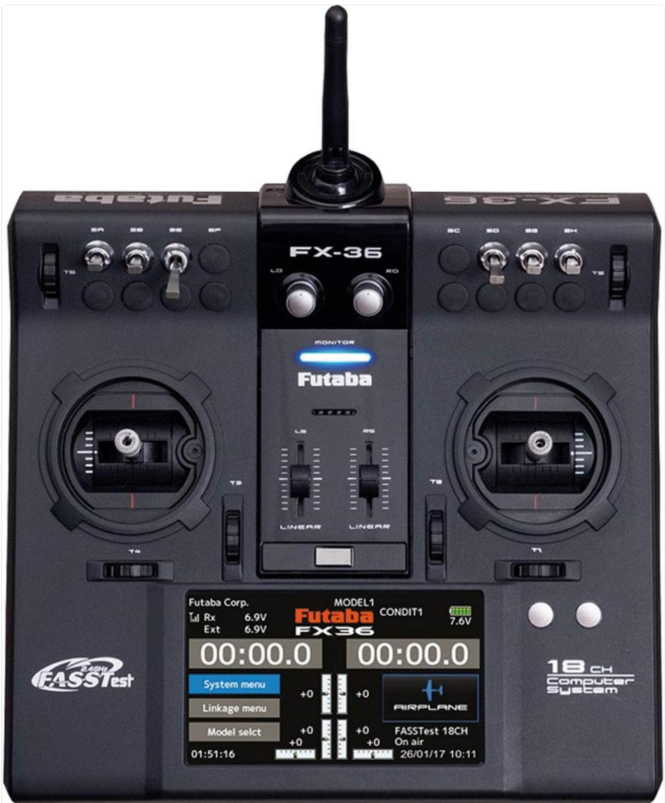
Figure 1: Front view of the Futaba FX-36 remote control system, showcasing the large color touch screen and dual control sticks.
