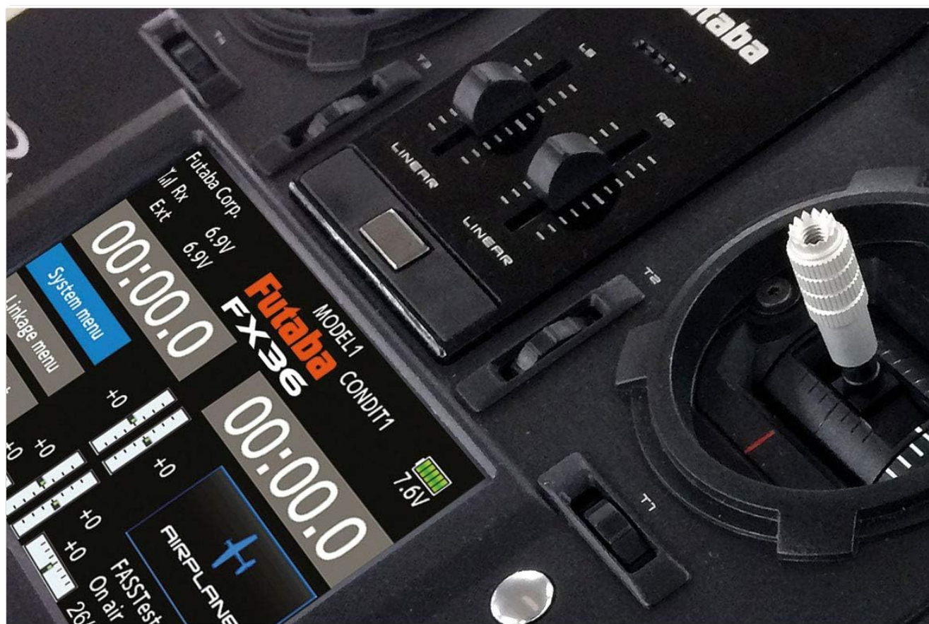
Figure 2: Detail of the FX-36 touch screen interface and linear control sliders.
