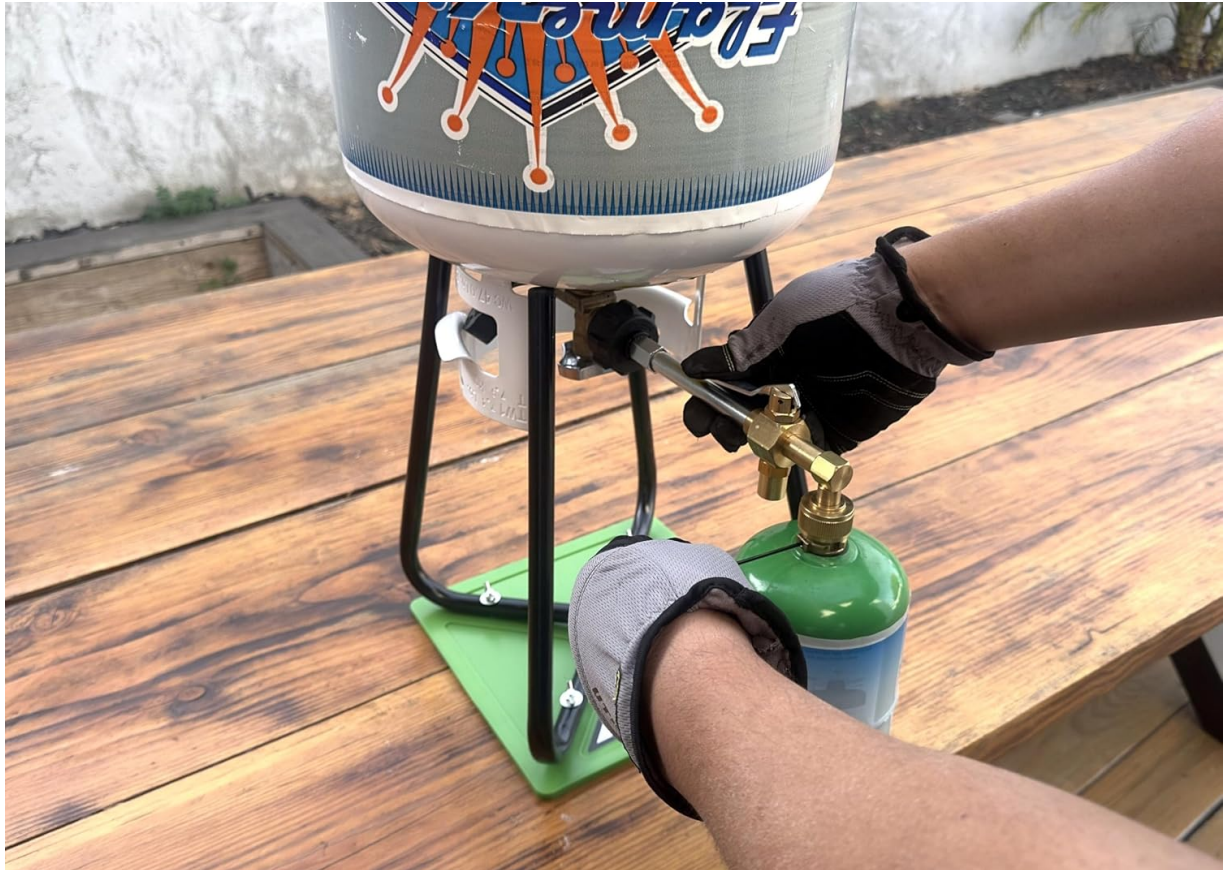
Figure 5: Connecting the 1LB cylinder to the refill adapter.
