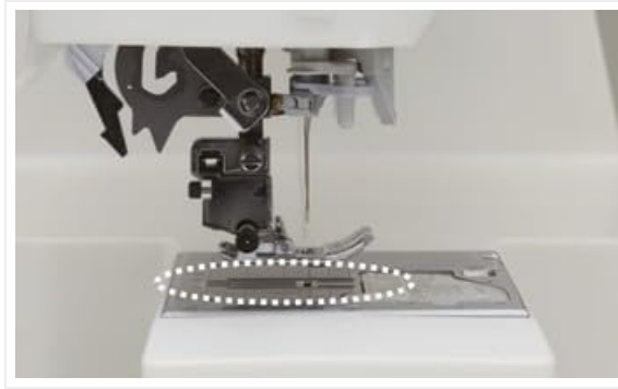
Close-up view of the needle, presser foot, and feed dog mechanism on the Juki HZL-NX7 sewing machine.
