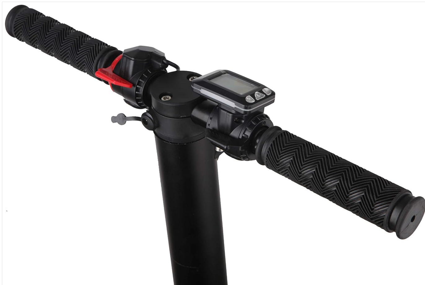
Figure 2.2: Handlebar and Display. A detailed view of the scooter's handlebar, showing the grips, brake lever, and the digital display unit which indicates speed, distance, and battery level.
