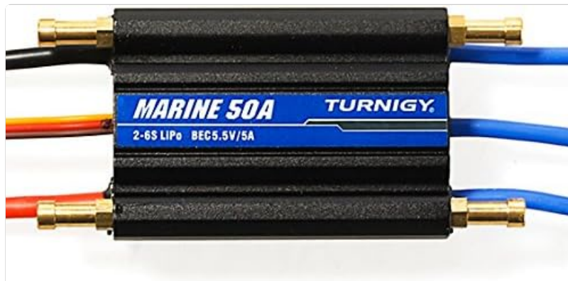
Figure 1: The Turnigy Marine ESC 50A, showing its compact design and connection points.
