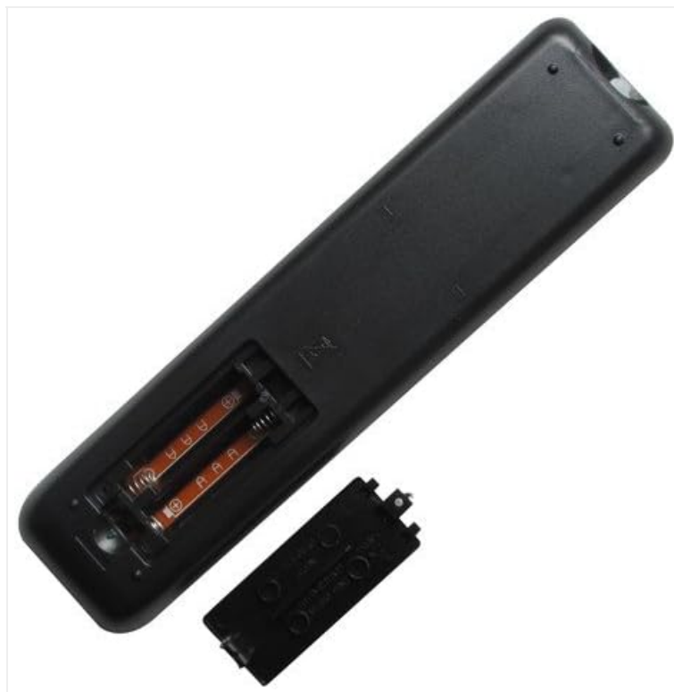
Figure 2: Battery compartment with cover removed, showing battery placement.
