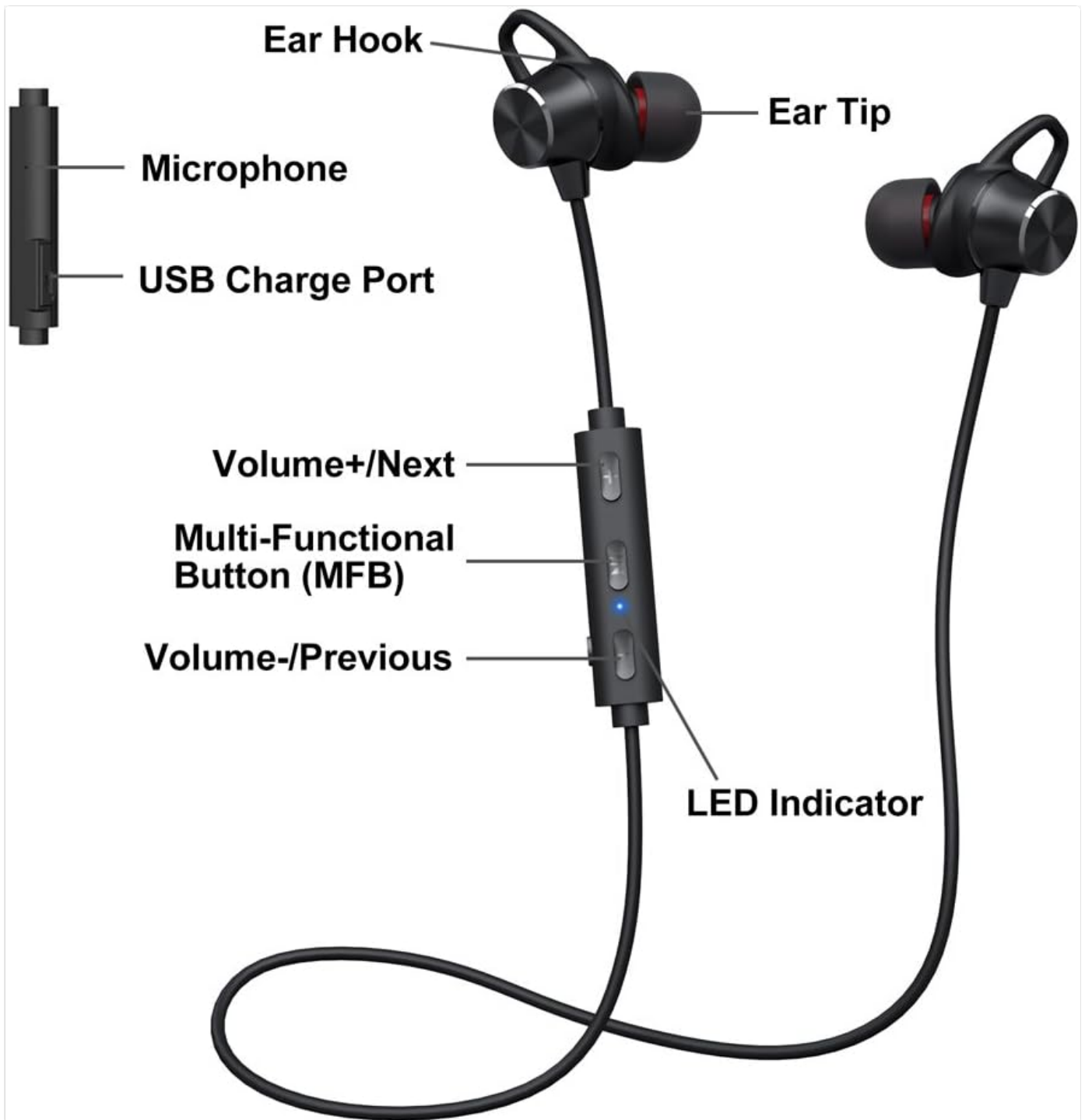
Figure 2: Key components and controls of the headset.
