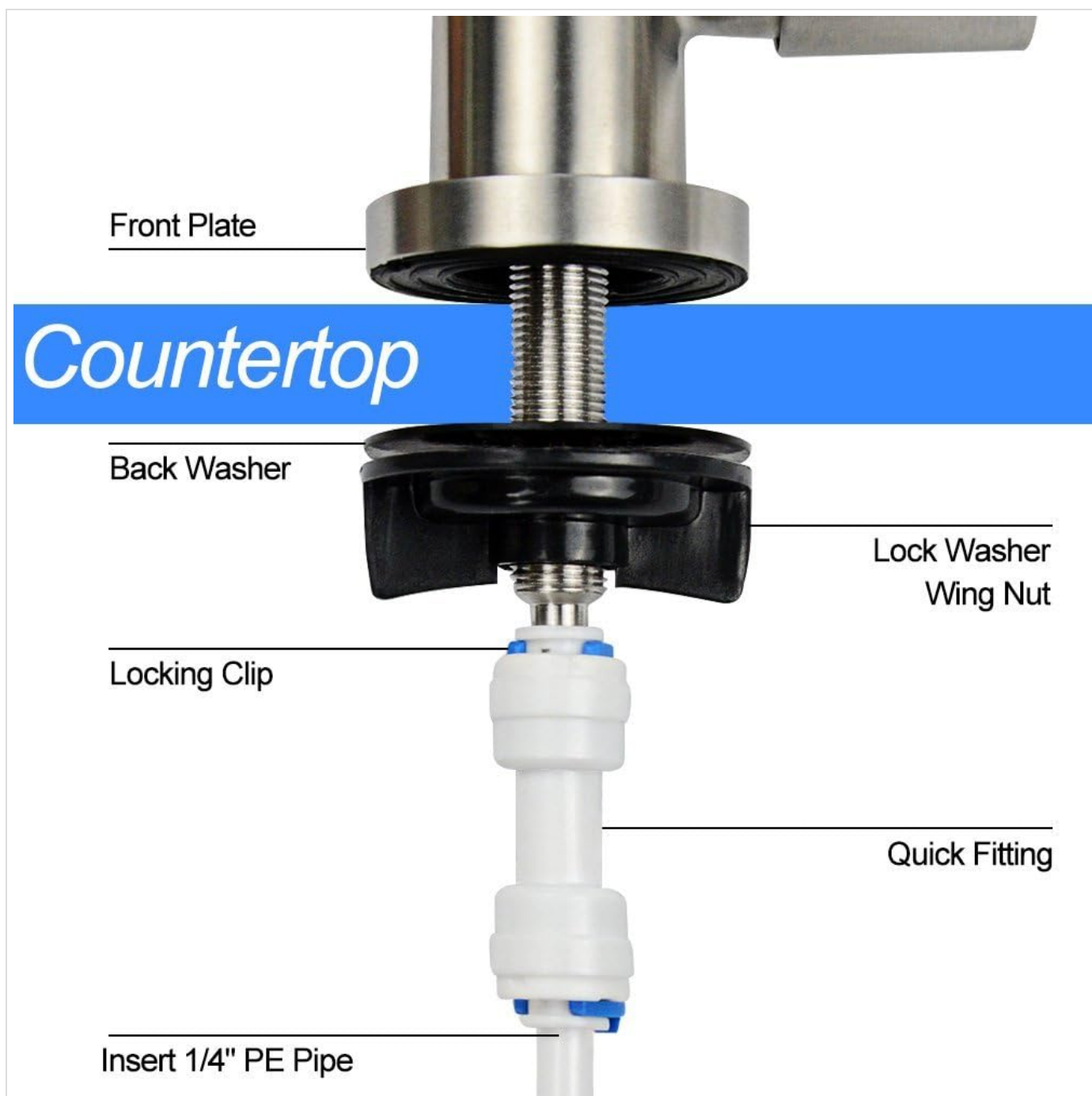
Image 4: Detailed diagram of faucet mounting hardware and water line connection.
