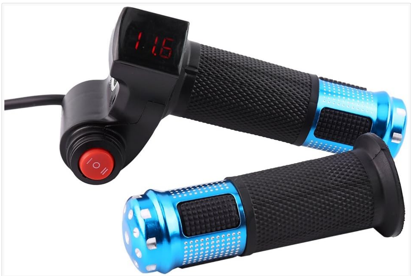
Figure 4: Close-up view of the LED display, which shows the current battery voltage.
