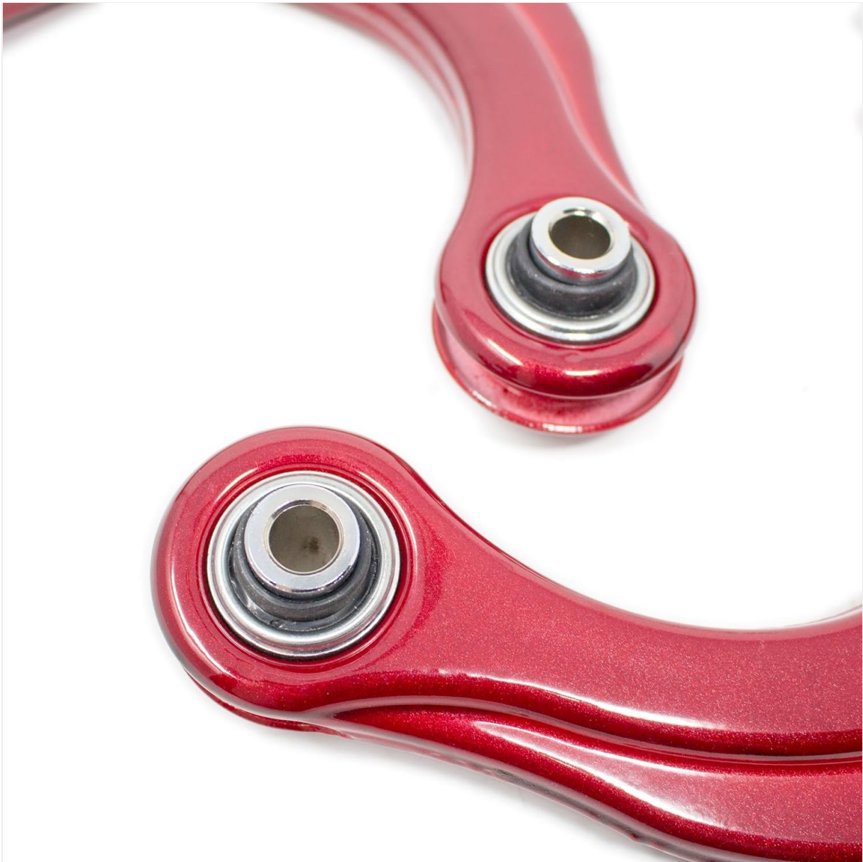
Image 6.1: A close-up view of the spherical bearing integrated into the Godspeed AK-038-F camber arm, highlighting its robust design for articulation and durability.
